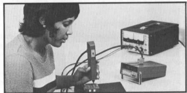
Fig. 6. The J6505 LED Test Probe being used for incoming inspection of light-emitting diodes by Brenda Bryant.
